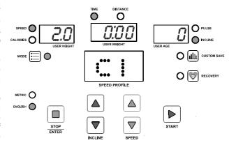
When the computer is in save program status, the "CUSTOM SAVE" button will blink slowly. Press the button to save this program or press the STOP/ENTER button to delete the program and return to POWER ON status.
